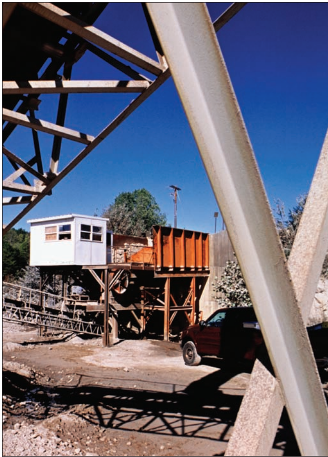
The basic plant-production flow at Highland Sand Co. begins with the primary jaw crusher and then onto a Metso 5x14 double-deck screen.
